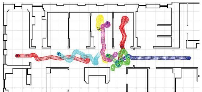
Stage is designed to support research into multi-agent autonomous systems, so it provides fairly simple, computationally cheap models of lots of devices rather than attempting to emulate any one device with great fidelity.
